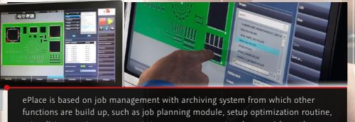
ePlace is based on job management with archiving system from which other functions are build up, such as job planning module, setup optimization routin setup list generator, component storage management and more. A barcode reader is used for feeder setup and replenishment, which is the quickest and safest way to assign a component to a feeder.
