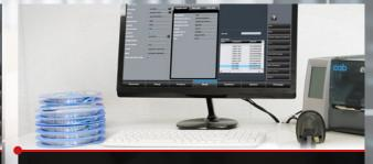
The new eMIS Management Software Suite for SMT production includes functions for job planning, feeder setup optimization, stock management, traceability, operational data analysis, line management and much more. With eMIS, managers and operators can keep track of actual, future and past production. Flexible interfaces simplify integration into your existing ERP and MES environment.
