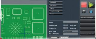
Eez-Technology allows easy and intuitive control of highly complex processes used in high-mix SMD production environments. It combines state-of-the-art .net software technology and an integrated database with a clear and structured graphical user interface. This interface visualizes in real time actual production runs and gives clear information about the current status.
