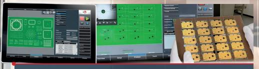
ePlace is based on job management with archiving system from which other functions are build up, such as job planning module, setup optimization routine, setup list generator, component storage management and more. A barcode reader is used for feeder setup and replenishment, which is the quickest and safest way to assign a component to a feeder.
